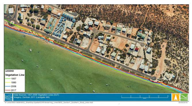
FIGURE 5-3 SECTION 1 SHORELINE MOVEMENT: 1957, 1990, 2006 AND 2017
