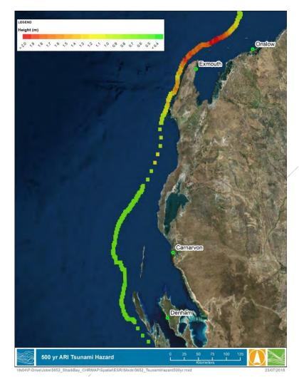
FIGURE 4-8 PREDICTED TSUNAMI WAVE AMPLITUDE AT 100M DEPTH CONTOUR FOR 500-YEAR ARI (GEOSCIENCE AUSTRALIA, 2009)
