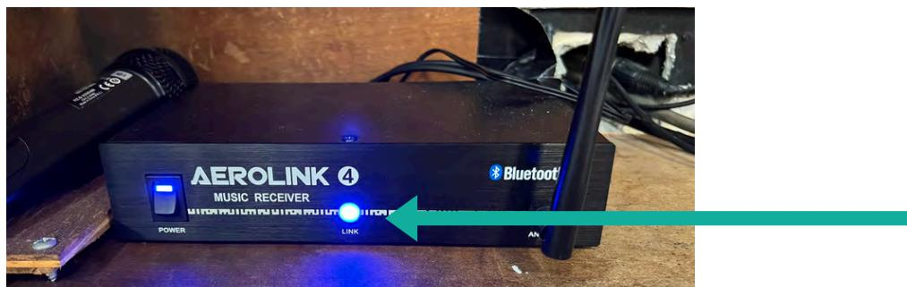
3. On the Aerolink Bluetooth box, press the center button (as seen in the picture) to make the device ready for pairing. If it is ready to pair, it will be flashing. On your device, go to your Bluetooth settings and pair with AEROLINK4.
