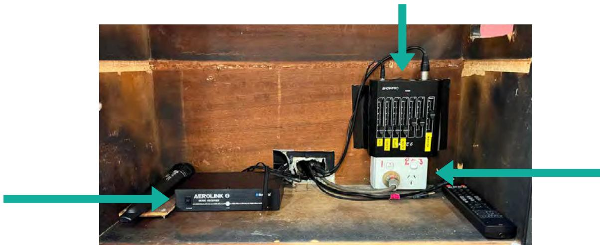
3. On the Aerolink Bluetooth box, press the center button (as seen in the below picture) to make the device ready for pairing. If it is ready to pair, it will be flashing. On your device, go to your Bluetooth settings and pair with AEROLINK4.
