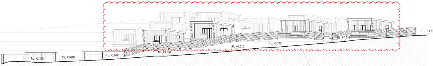
1 STREET ELEVATION FROM DENHAM ROAD WITH FENCE 1:250
