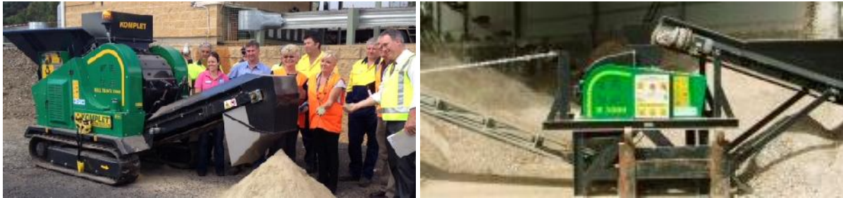
Example of dedicated glass crusher (Komplet M5000)
