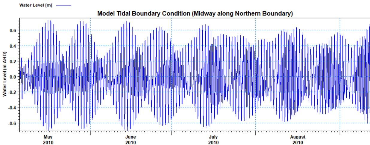
FIGURE 4-3 MODEL TIDAL BOUNDARY CONDITIONS (MIDWAY ALONG THE NORTHERN BOUNDARY)
