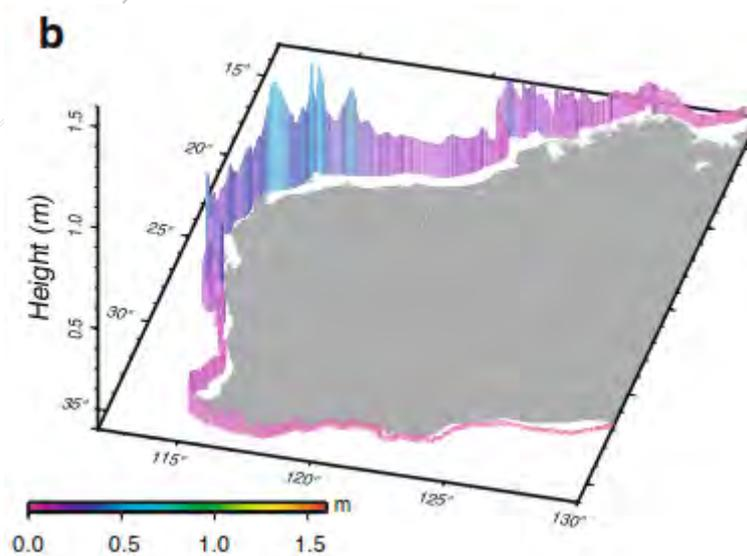
FIGURE 4-9 PREDICTED TSUNAMI WAVE AMPLITUDE AT 50M DEPTH CONTOUR FOR 500-YEAR ARI (BURBIDGE ET AL, 2008)
