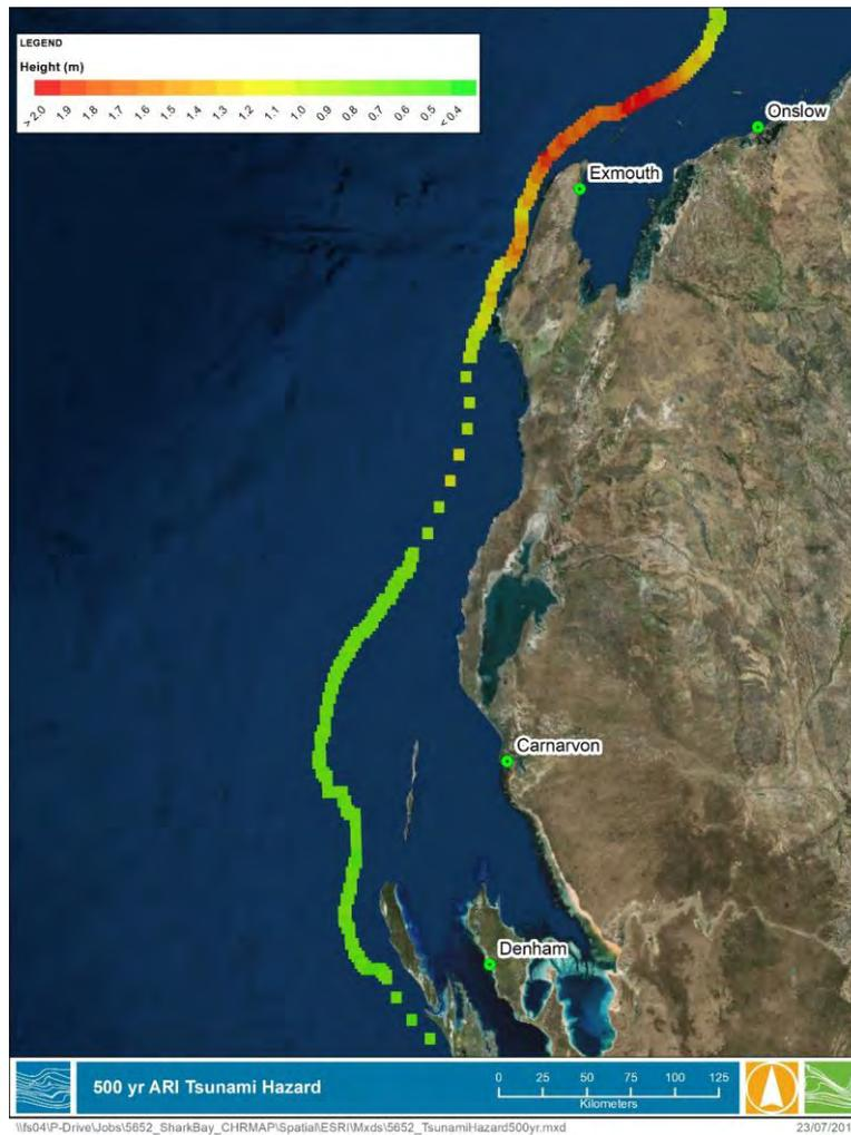
FIGURE 4-8 PREDICTED TSUNAMI WAVE AMPLITUDE AT 100M DEPTH CONTOUR FOR 500-YEAR ARI (GEOSCIENCE AUSTRALIA, 2009)
