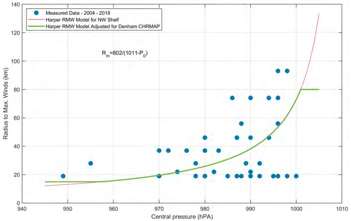
**FIGURE 4-4 NON-LINEAR FIT ON RADIUS TO MAXIMUM WINDS VERSUS CENTRAL PRESSURE FOR CYCLONES PASSING WITHIN 500KM OF DENHAM**
