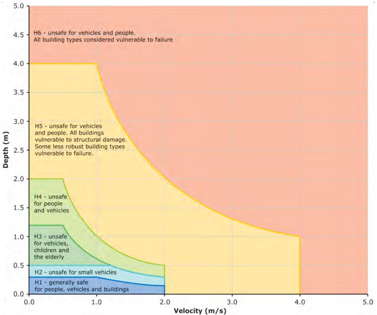
FIGURE 3-2 FLOOD HAZARD CURVE (SMITH ET AL, 2014)
