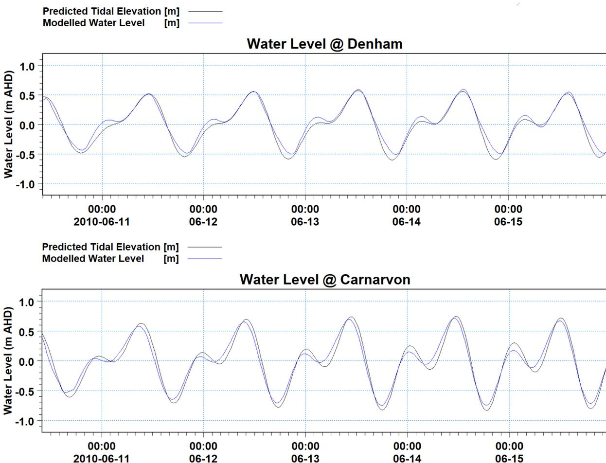
**FIGURE 4-7 TIME SERIES OF PREDICTED AND MODELLED WATER LEVELS FOR A TIDE ONLY SIMULATION AT DENHAM & CARNARVON**
