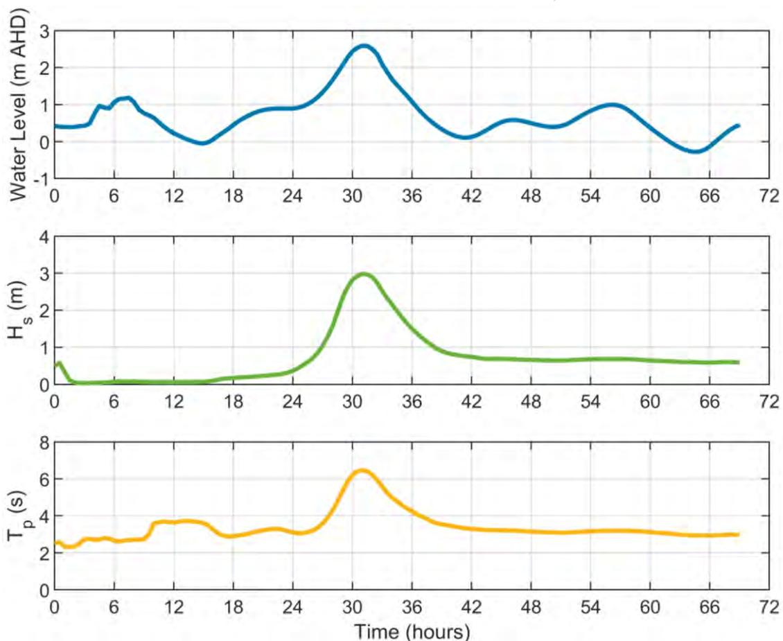
FIGURE 5-1 TIME SERIES OF DESIGN WATER LEVEL AND WAVES APPLIED IN SBEACH (STORM 1 OF 3)
