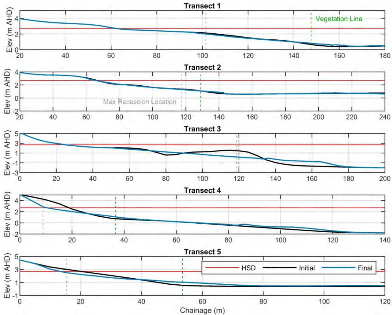
**FIGURE 5-2 SBEACH RESULTS FOR EACH TRANSECT, REPRESENTING EACH COASTAL SECTION**
